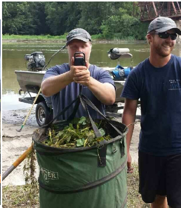
Water chestnut in a laundry bag and lawn bag weighed using a digital hanging scale. It is recommended that scales with at least a 50 or 100 pound capacity are used.
