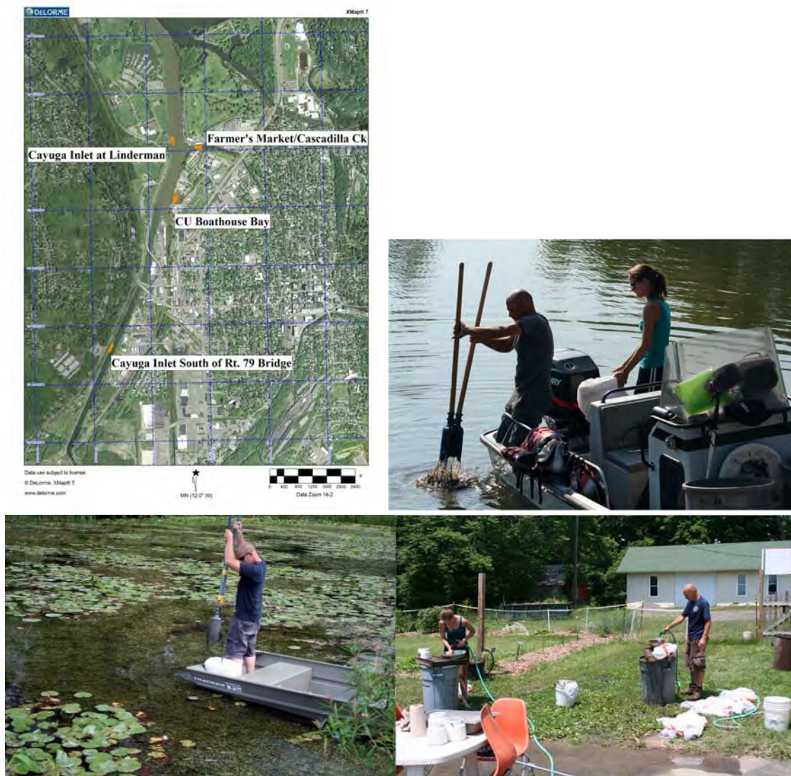
Figure 6. Map above shows the four locations in the Cayuga Inlet where we routinely conduct sediment core removals while the three additional photos show sample collection and processing.
