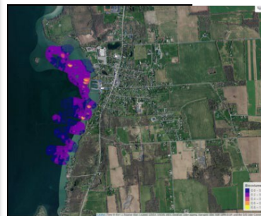
BioBase survey sites in 2021 across 6 waterbodies and example maps of data processed by BioBase, and displayed using R showing biovolume and bottom hardness at Union Springs, on Cayuga Lake.
