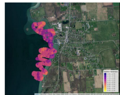
BioBase survey sites in 2021 across 6 waterbodies and example maps of data processed by BioBase, and displayed using R showing biovolume and bottom hardness at Union Springs, on Cayuga Lake.
