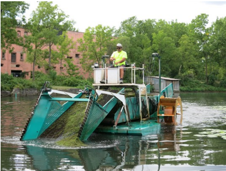
An aquatic vegetation harvester cutting through starry stonewort. Keuka Lake, 2020.
