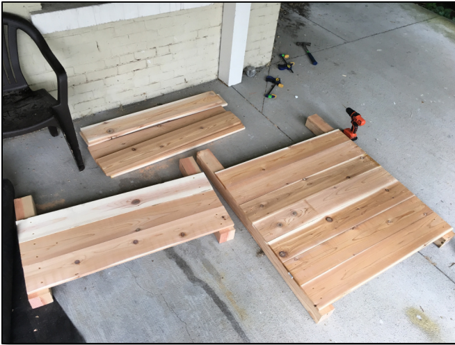
1. Assembled front (left) and back (right) panels
